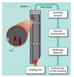
Figure 2: Drying process for the Quiver (schematically)
