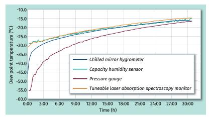
Figure 3: Validation of the Tuneable Laser Absorption Spectroscopy Monitor
