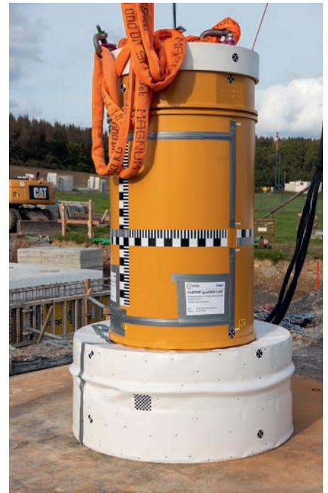
Test specimen after the 9 m drop.
