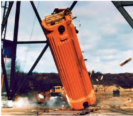
BAM test site in Lehre in 1978: Initial 1:1 drop tests with a CASTOR® 1a prototype.
