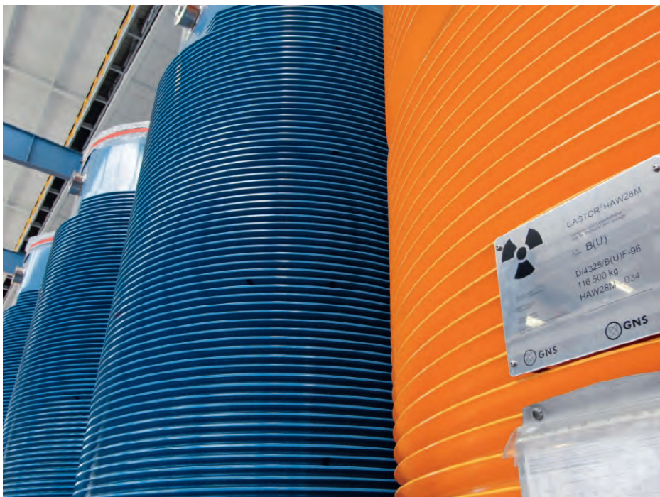
A CASTOR® HAW28M for retrieval of vitrified reprocessing waste next to CASTOR® V casks for spent fuel assemblies in the GNS cask production in Mülheim.
