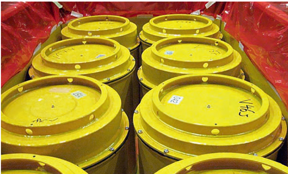
Overpacks with evaporator concentrate drums placed in type IV Konrad containers.
