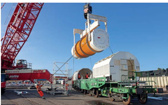
Fig. 7. Arrival of the MV Pacific Grebe at the Port of Nordenham. Transferring a CASTOR® HAW28M from the MV Pacific Grebe onto a railroad car.
