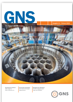
Title: Installation of the primary lid of a CASTOR® 1000/19 for irradiated fuel assemblies of the Czech nuclear power plant Temelin in the GNS cask assembly in Mülheim.
