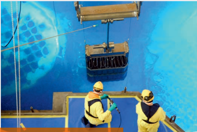
Underwater dose rate measurement on a loading magazine at KKG.
