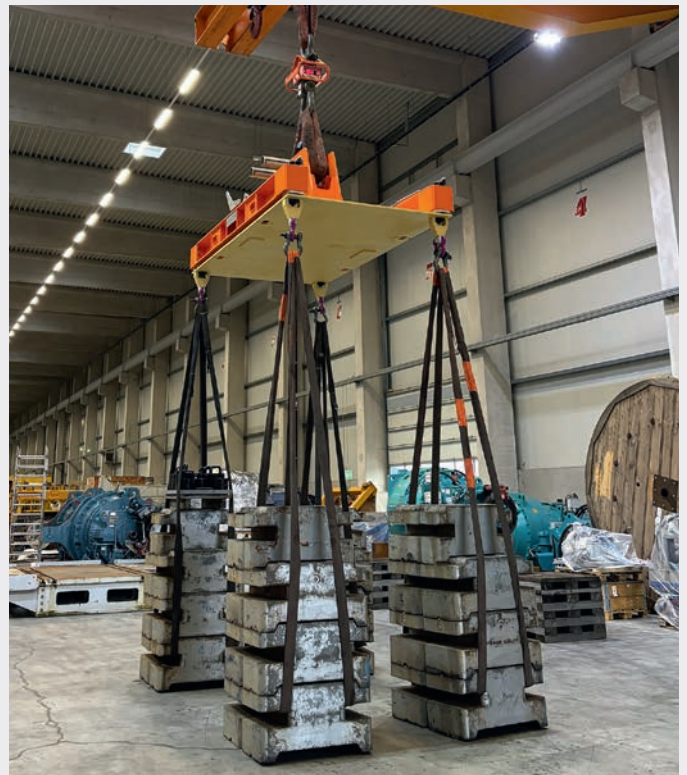
The KC spreaders have passed the 30-tonne overload test with flying colours.
