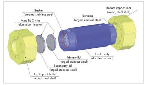
Fig. 3. CASTOR<sup>®</sup> V/19 in transport configuration (with impact limiters).
