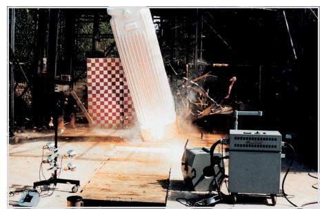
Fig. 2. Drop test of CASTOR® IA.
