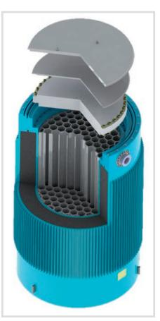
Fig. 8. Schematic diagram of a CONSTOR® cask for hexagonal fuel assemblies.
