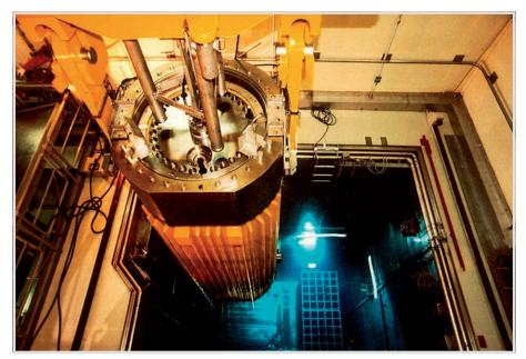
Fig. 4 CASTOR<sup>®</sup> Ib after loading.
